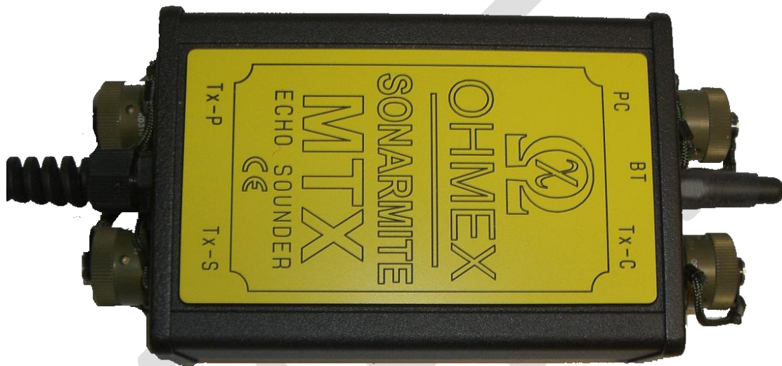
SonarMite MTX multiple beam echo sounder
